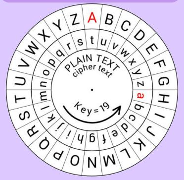
On this example, the key is 19, meaning that the inner circle has been moved 19 times to the right
